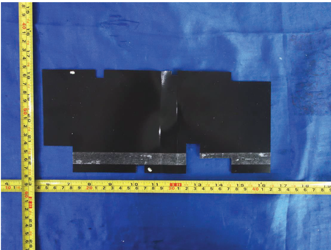
Figure 12. Mylar sheet around power board
